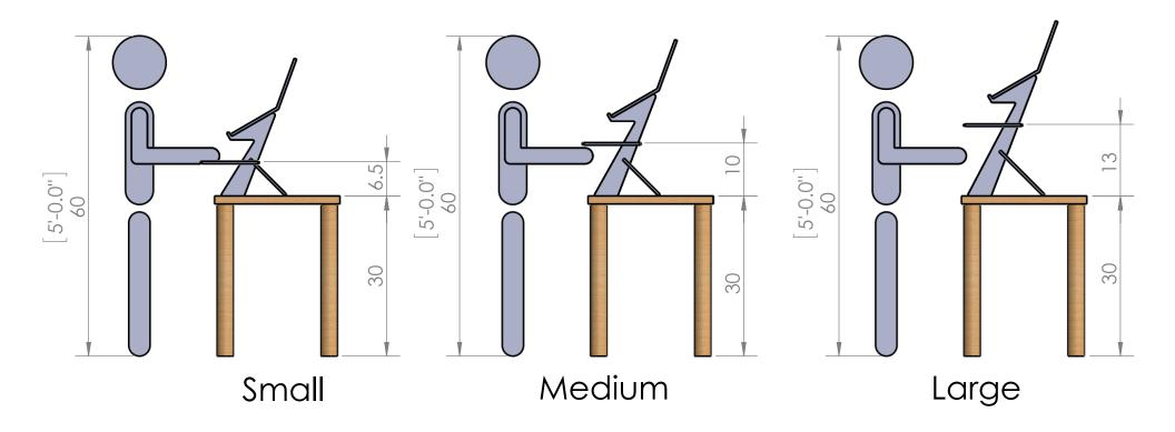
Note: Keyboard tray can move up or down by 2 inches in 1 inchincrements. Image shows tray at mid point.
